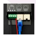
7. If cascading/daisy-chaining multiple units, use an RJ45 cable to connect to between one controller unit and another (please refer to the wiring diagram - pq2).
